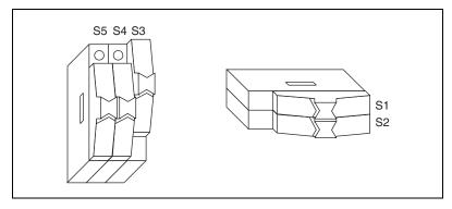
Figure C-1. General-Purpose Switch Configuration for the SCB-68 Terminal Block
